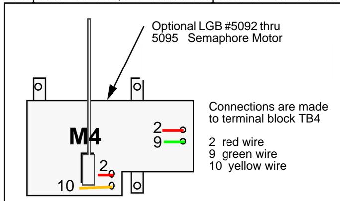
Figure 28—Wiring Alternate Semaphore Motor
